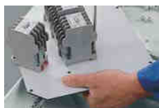
Mounting plates for the installation of electrical devices
