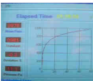
Test temperature curve in accordance with DIN 4102
